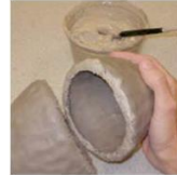
Add slip to the scored edges on both sides.
